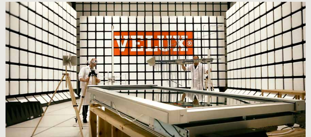
Tested for the effect of unwanted electromagnetic fields, interference, radio waves and noise in Northern Europe's only audio centre.
