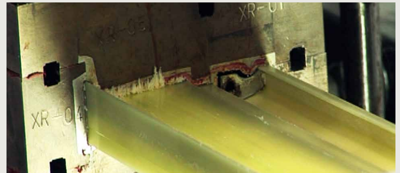
A pultrusion process moulds the composite and creates an exact form.
