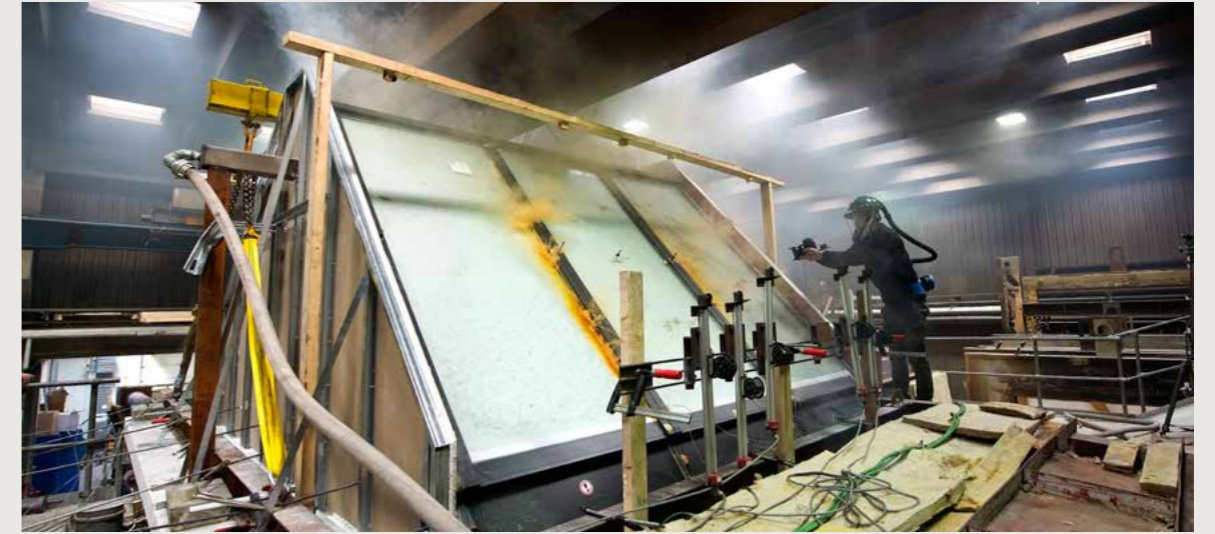
Pyrotechnical testing. Glazing unit and profile are able to sustain more than 900° C for at least 30 minutes
